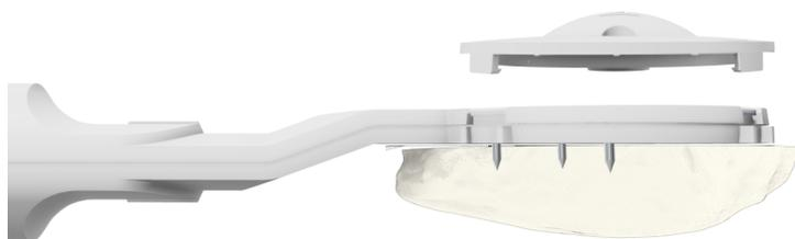
Mark the position of the sensor at the indents using preferred technique, e.g. with methylene blue (Figure 27). This should allow for easier positioning of the sensor in the same place, for subsequent readings.
