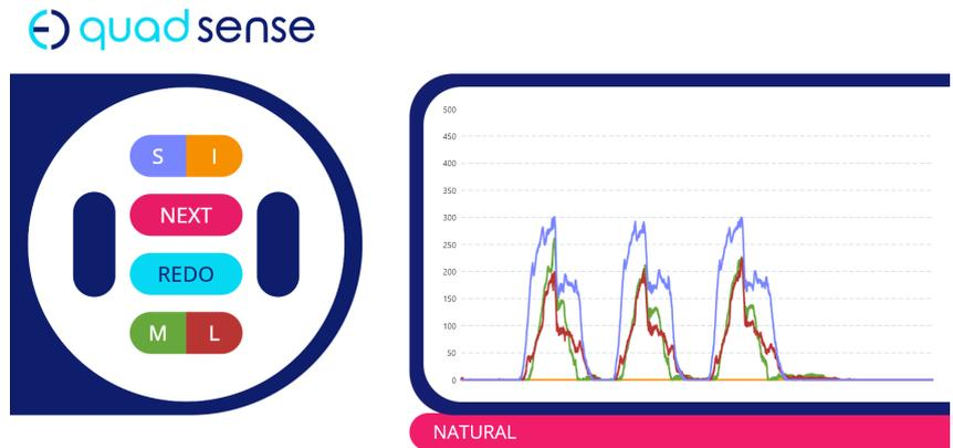
The y axis is relative load, and the x-axis is time. If the leg is moved through flexion extension consistently three times, there should be 3 distinct peaks of similar height.
